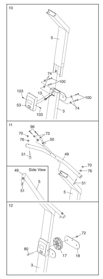
Pull the upper cable (B), which is attached inside of the Mech Assembly (6), up between the Upright (3) and the Pulley Plate (18).
